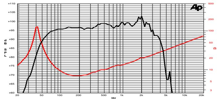
Frequency Response on 90 Lt @ 48 Hz Vented Box @ 1W, 1m
