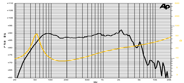
Frequency Response on 25 Lt @ 45 Hz Vented Box @ 1W, 1m Free Air Impedance
